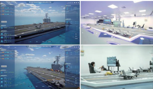
图 6 航空保障作业数字孪生仿真推演试验平台 Fig. 6 Aircraft carrier aviation support operations digital twin simulation and deduction test platform
