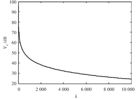
Fig.3 Relation curve of the shaft-ground voltage and the gain
