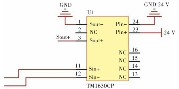
(b) Circuit module of isolation transmitter
