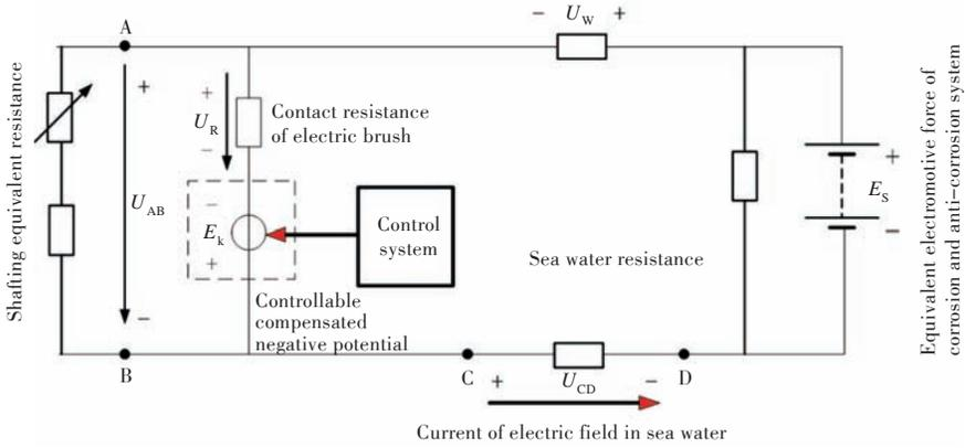
Fig.1 Schematic diagram of shaft system with compensation circuit
