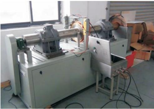
Fig.7 Scale model of ship shaft system
