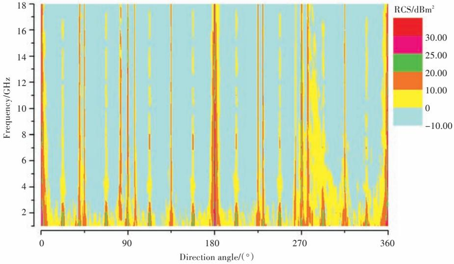
Fig.2 RCS distribution of mast in different frequencies and angles
