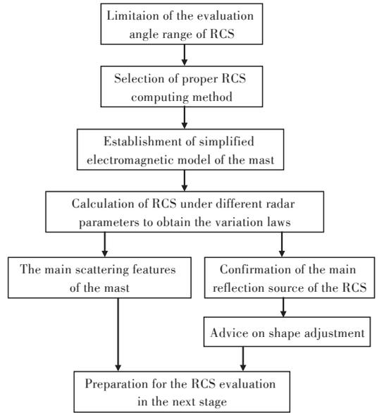
Fig.9 The evaluation process of stealth shape
