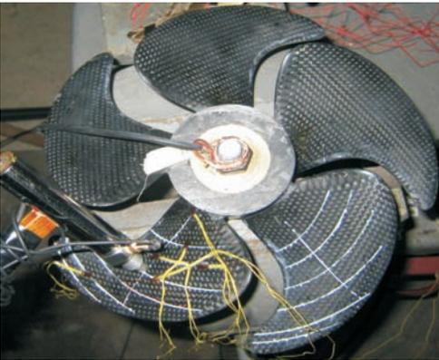
(a) Photo of carbon fiber propeller
